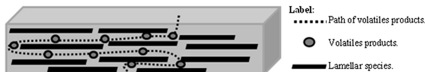
Fig. 3. Schematic representation of the effect of the physical barrier provided by the lamellae organoclay in a polymeric matrix.
