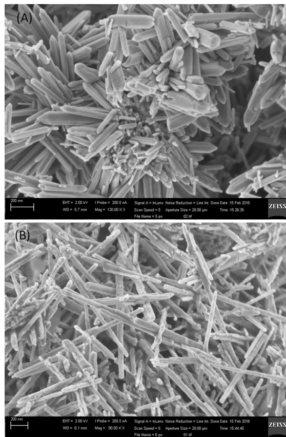
Fig. 2 FE-SEM images of ZnO nanoparticles. a Sonication for 10 min (nanoflowers). b Sonication for 40 min (nanoneedles)
