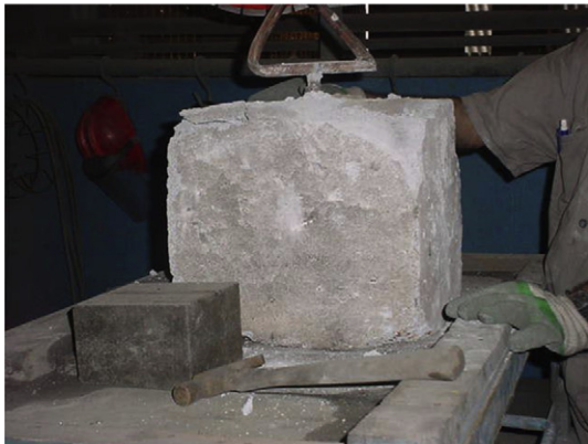
Fig. 10. Aspect of molded refractory blocks after industrial convective drying/heating curve.
