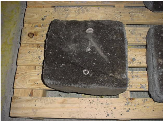
Fig. 13. Aspect of molded refractory blocks, with ceramic coating on, following industrial convective drying/heating curve.
