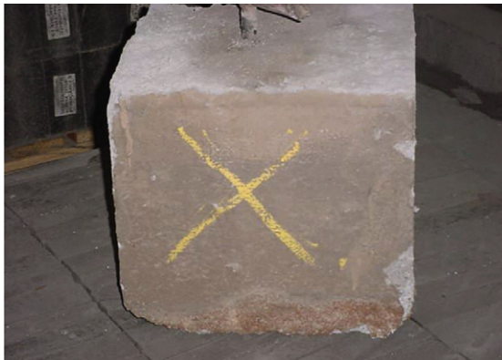
Fig. 13. Aspect of molded refractory blocks, with ceramic coating on, following industrial convective drying/heating curve.
