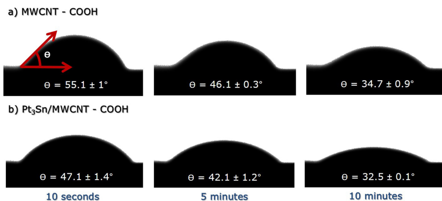
Figure 2. Contact angle images of water on a) MWCNT-COOH, b) Pt 3 Sn 2 /MWCNT-COOH at 1 min, 5 min and 10 min. T = 20 °C.
