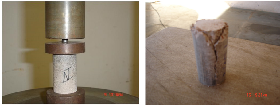
Fig. 4. Image of the TS before (left) and after compression test exhibiting prismatic fracture (right).
