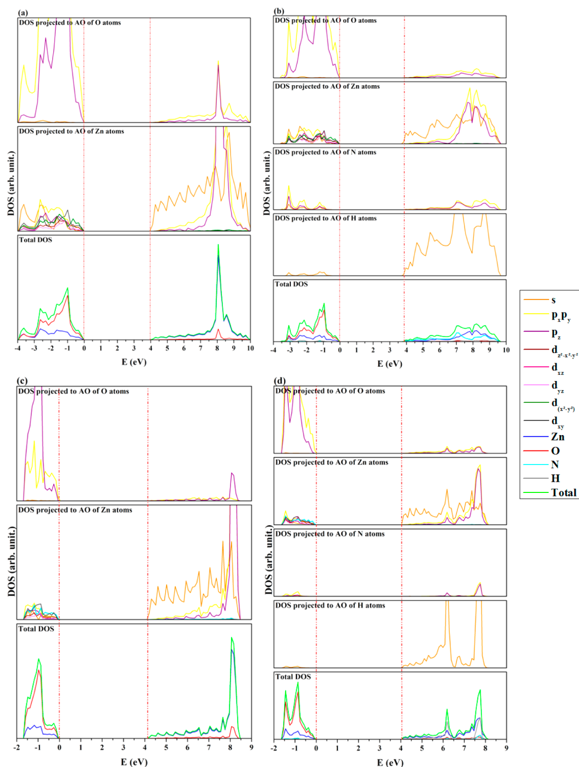
Figure 3. Density of states of (10, 10) nanotube (a) bare and (b) with 10-rows of \text{NH}_3 molecules adsorbed and (20, 0) nanotube (c) bare and (d) with 10-rows of \text{NH}_3 molecules adsorbed.
