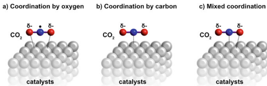
Fig. 6 Representative scheme of possible adsorbed \text{CO}_2 species on the surface of a catalyst
