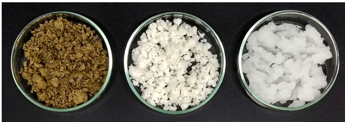
Fig. 2. Images of cellulose pulp after extraction by organosolv pulping, bleaching, and TEMPO-mediated oxidation (from left to right).
