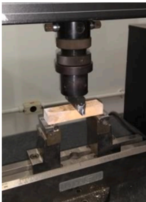
Fig. 1. Three-point flexural strength test.
