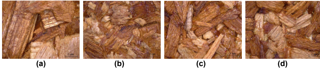
Fig. 1. Surfaces of homogeneous (T1) and heterogeneous (T2) particleboards (8x magnification): (a) surface of T1, (b) surface of T2, (c) core of T1, and (d) core of T2 samples.
